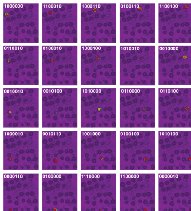
Figure 6. Selective Raman mapping of 25 BCRs. The binary codes refer to the tagged styrene content according to Figure 1 and ref 29b. The correlation thresholds were adjusted to ensure classification with 100% confidence and varied between 0 and 90%. When the correlation threshold was fixed at 90%, the beads appeared red.
